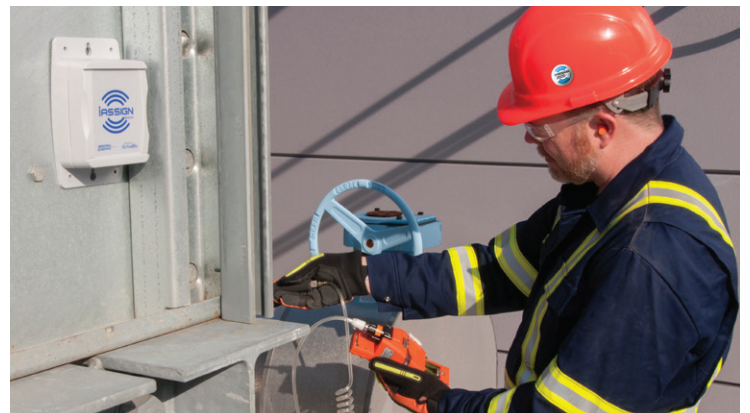
iAssign Beacons – Automatically assign location names to Ventis Pro5 Multi-Gas Monitors based on proximity, helping safety managers see where hazards occurred and who was involved.
